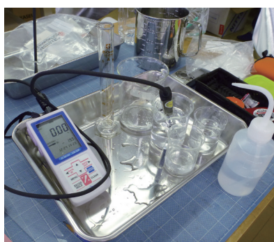
図6 電気伝導率計（塩分濃度計測）（TOKO, CT-27112B型） Fig. 6 Electrical conductivity-measuring device (salinity measurement) : TOKO CT-27112B
